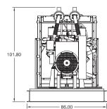
Drawings based on standard open power 480 volt standby generator. Lengths may vary with other voltages. Subject to change without notice. Sound data as measured at 23 feet (7 meters) in accordance with ISO 8528-10 at standby rating.
