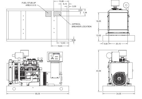
Drawings based on standard open power 480 volt standby generator. Lengths may vary with other voltages. Subject to change without notice. Sound data as measured at 23 feet (7 meters) in accordance with ISO 8528-10 at standby rating.
