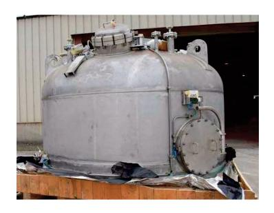
3V Tech SPA Filtro 1000 FPP/FF Filter Agitated Nutsche Filters. 316 Stainless Steel. Capacity 10,946.99 square feet. Internal rated 50 psi / FV at 212 degrees F. 10.17 Square meter filtering area. 10.79 Cubic meter product volume. Hydraulic power pack with 7.5hp, xp motor. 3/60/460 Volt.
