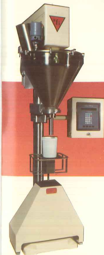
Fig. 8 Model BS-300 Semi-automatic Filler for Rigid Containers
