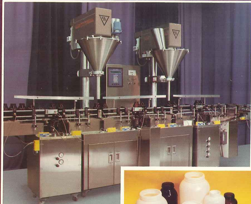
Fig. 14 Versatile net weight filling system stores 100 different product/container combinations in Cerebus II memory. Fills chemical reagents from 1 to 1000 grams.
