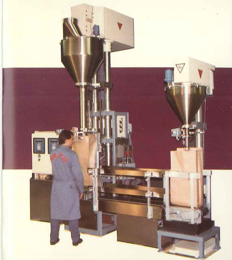
Fig. 7 Model BD-300 Semi-automatic Bulk & Dribble Filler for filling large open mouth bags with a powdered food product. Designed for several bag sizes for net weights of 25 to 100 lbs., it is capable of producing 50 lb. bags within ½-ounce up to 600/Hr. Bags are manually hung, bottom up filled and jogged during the bulk fill cycle. A dust collecting shroud moves with the bag lift. A powered conveyor transports bags to the dribble fill station for exact top-off.
