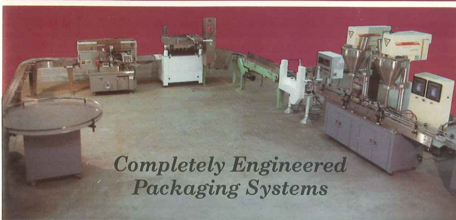
Fig. 14 Versatile net weight filling system stores 100 different product/container combinations in Cerebus II memory. Fills chemical reagents from 1 to 1000 grams.
