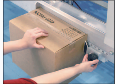
Wexform 615T tool-less length adjustment
