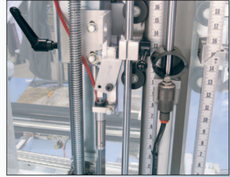
Wexform 615T tool-less height adjustment system
