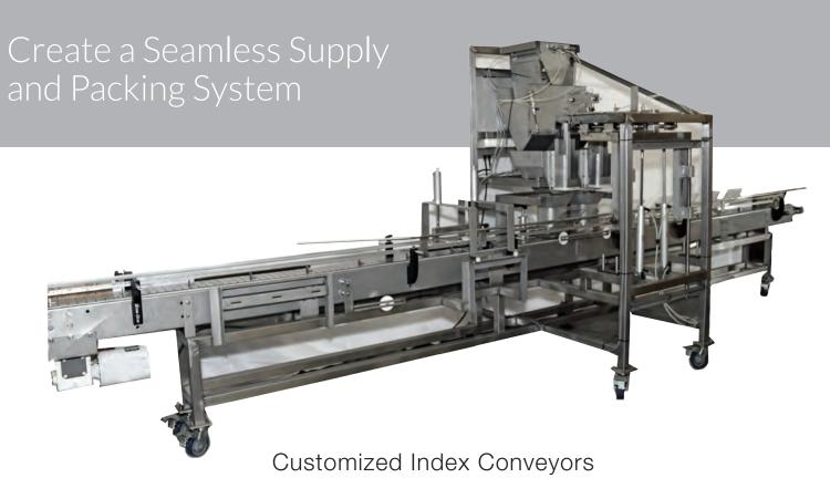
Ohlson's customization and engineering capability provides seamless integration of the packaging process when required. Custom Indexing conveyors can automatically present the containers under the single or multiple discharge chutes from the scales and move them downstream for final closing and/or labeling. From there the container is ready for manual or automatic case packing to complete the process.
