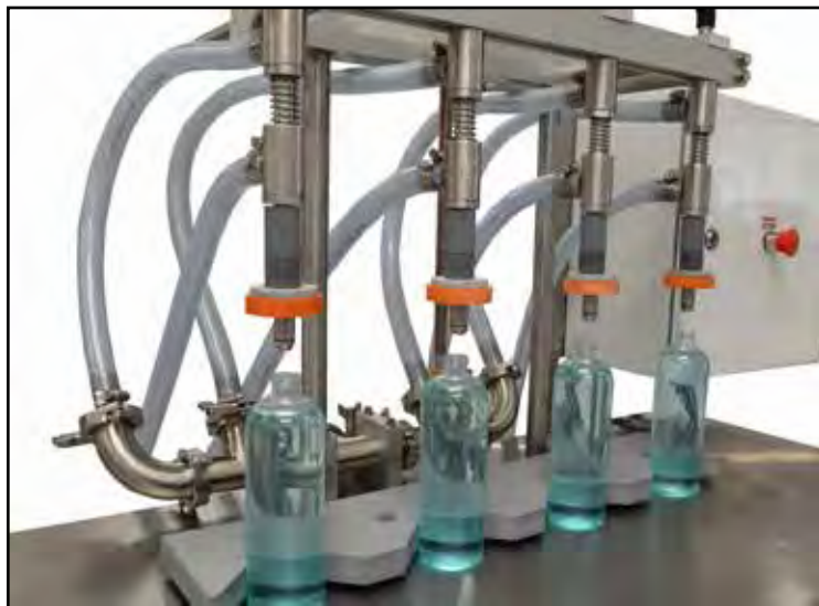
Accutek Single O-ring Overflow Nozzles
