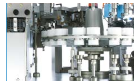
Servo lifting station for print registration and filling station
