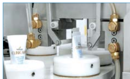
Tube pressing, emboss coding and discharge stations
