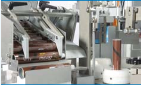
Tube feeding conveyor – chute – rotary machine table
