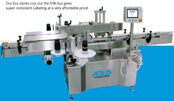
The Eco Panel is shown with optional extended conveyor, PLC control with a Color touchscreen, Servo controlled top hold down belt, servo controlled feed screw, Wrap Belt for round containers, and a Prism Roller aligner.
