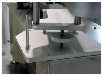
A nice touch on the Aesus Eco labelers is the Tilt adjuster with graduated scale to fine tune the angle of the label head to match the container precisely.
