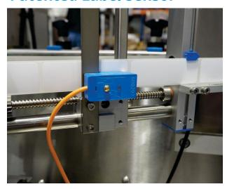
Patented Inductive label sensor eliminates the need to play with photo electrics which can accumulate dust.
