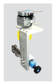
For speeds up to 120 per minute the Star Prism holds the container, spins it, (aligns it to a mark if needed), applies the label(s) and indexes it.
