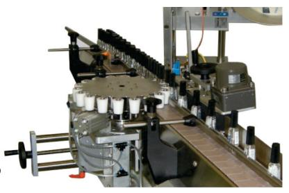
Prism alignment is for long labels where perfect alignment is required, two labels (front and back) on the same roll, alignment of a handle etc. with the label.
