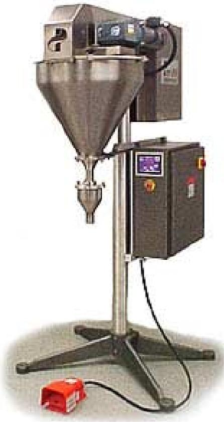
Precise encoded motion of the auger, peak power start and stop fill-cycle prevent auger slip and drive train wear from affecting the fill accuracy.
