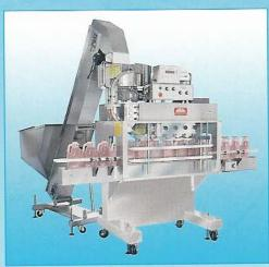
Available with optional Parts Elevator (shown) or Parts Escalator/Orienter/Feeder (not shown) both featuring waist-level loading.
