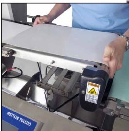
No-tools conveyor and belt installation for maximum uptime
