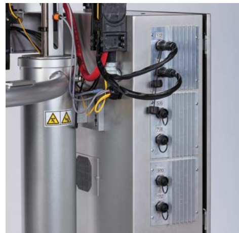
Six connection points for the 12 customer defined heat zones
