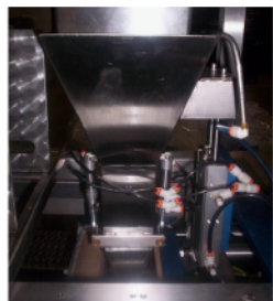
Transition Chute enters bag to prevent spillage and protect seal area
