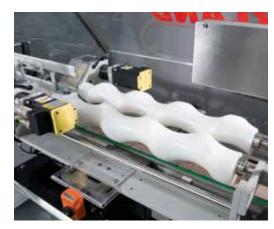
The 'Mercury' is the latest development in the Harland Linear Series of labelling systems. The system has been designed for production lines that have a high throughput speed requirement and the need for zero downtime production. This 4 or 2 station system can apply front and back labels to any shape of plastic bottle/container at speeds up to 250ppm and fits nicely in the Harland family of labellers, between the well proven 'Sirius' system and ultra high speed 'Titan'.
