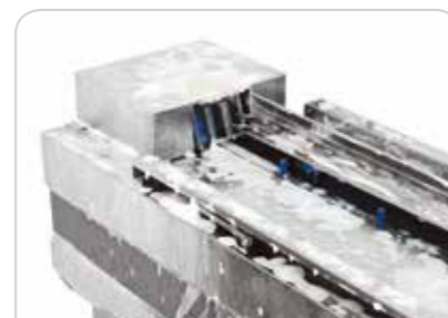
Infeed conveyor designed for easy cleaning
