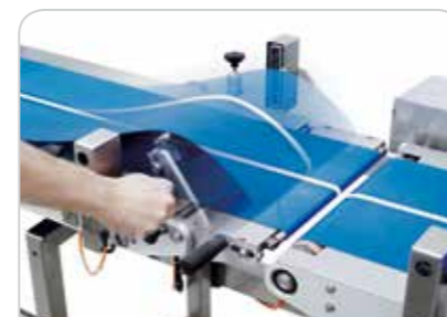
Easy feeding belt removing for cleaning
