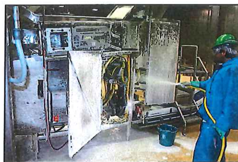
All components, both internal and external, have been chosen to withstand daily wash down
