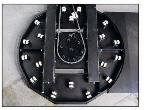
Heavy duty chain drive on turntable with 18 sets of double roller turntable supports.
