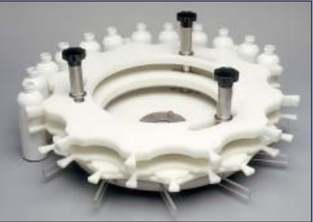
Bottom fill, open tube valves for viscous products
