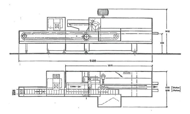
Output: . depending on carton size CARTOPAC CPS up to 250 cartons/min. CARTOPAC CPS-R up to 450 cartons/min.
