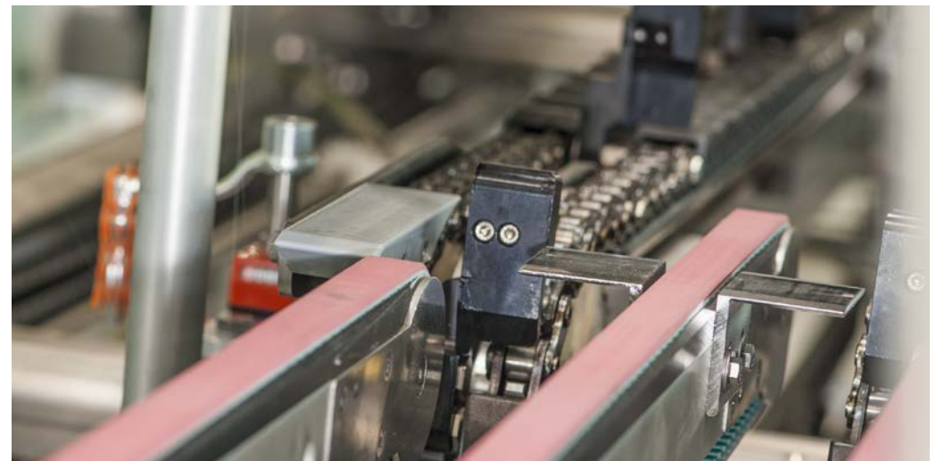
Conveyor and chain of pack forming unit
