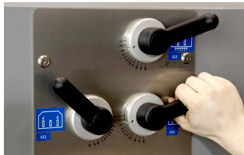
Easy adjustment of the air nozzles
