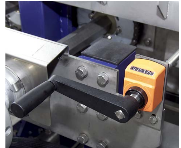
Crank for infinite adjustments (illustration above)
