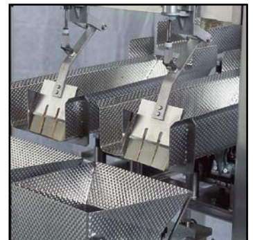
Cut-off gates guarantee fill accuracy
