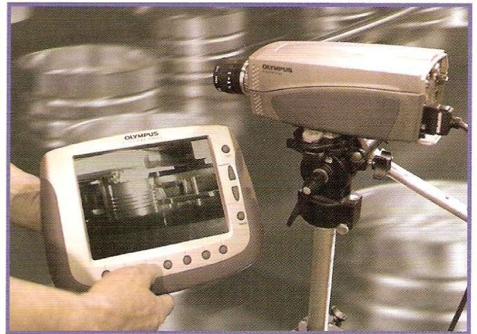
High speed portable video camera for analyzing fill characteristics
