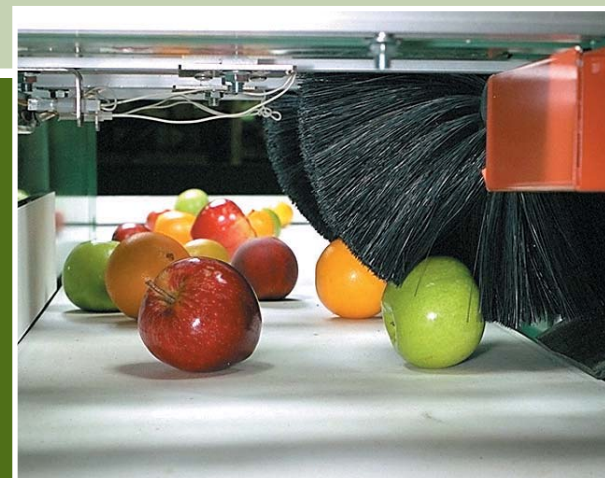
Gentle nylon brush letdowns deliver fruit to crossover conveyor
