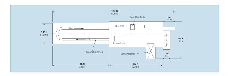
The OYSTAR Jones CMV® features heavy-duty construction, a patented belt closing system, positive carton opening and control, and self-cleaning vacuum lines. The ergonomically designed loading platform and many other production-proven features make OYSTAR Jones' vertical cartoners last for decades.
