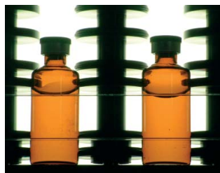
Background light in combination with Tyndall illumination.
