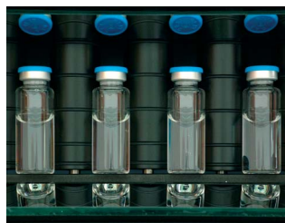
Two mirrors for bottom and cap inspection.
