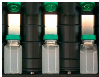
Special light adapted to suspensions.
