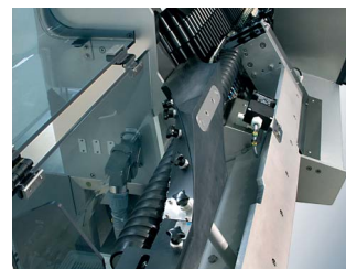
Syringe turning screw at infeed.
