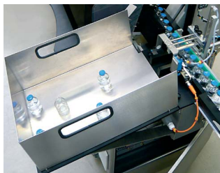
Separation of defects for bottles.
