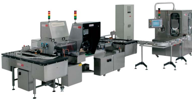
Integration with outside vial washer and buffer tables.
