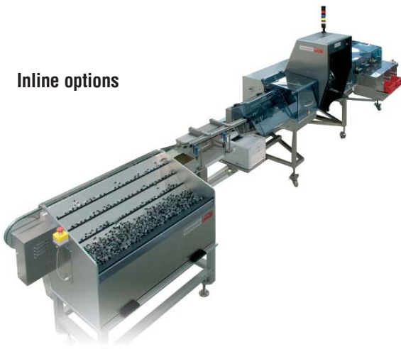
Bulk syringe feeding and orientation system in line with V90-AVSB.
