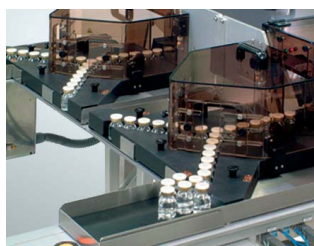
Y-Mag modules to separate two reject categories.
