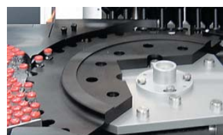
Tray unloader with segmented infeed starwheels.
