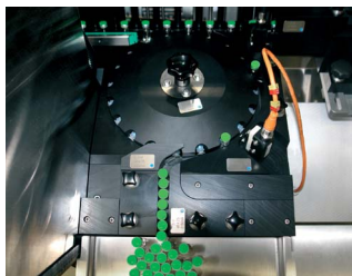
Separation of defects for ampoules and vials.
