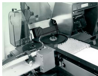
Infeed combination syringe/vial.
