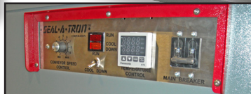
Standard Digital Temp Controls
