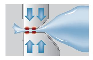
seal bar cut-off perforation pouch piercing knives
