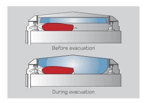
**Expansion Cushion** with **Snap-out Frame** reduces evacuation time by up to 30% and prevents wrinkles on the upper side of the package.
