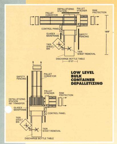
The Priority One Packaging Ltd. Low Level Bulk Container Depalletizing Systems are fully automatic. The modular design allows a system to be designed for the most demanding requirements. Tier sheets or inverted trays can be removed from between layers either manually or automatically These systems feature:
