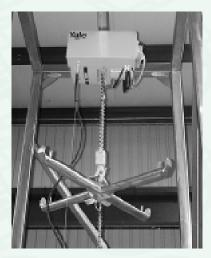
SHF-B Captures the bag loops between extended retainer tabs. Easy to change bags. Designed for use with manual and powered overhead hoists.
