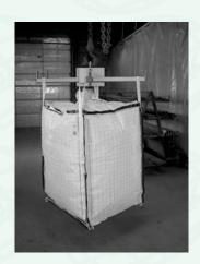
The SHF-B is a safe and economical solution to bulk bag handling. It features an easy on/easy off bag loop system and is equipped with a 5400 lb. screw type clevis.
