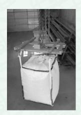
The unique engineering of the SHF-BL allows loop tension to be placed on the bag body vertically (as required for safe use) while holding the loop in a horizontal plane. The end result is superior loop tension and greatly reduced headroom.
