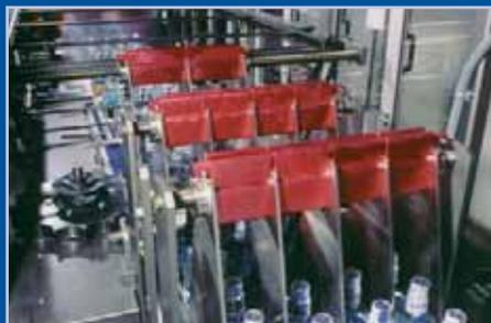
Infeed Conveyor with Color Coded Spacers
