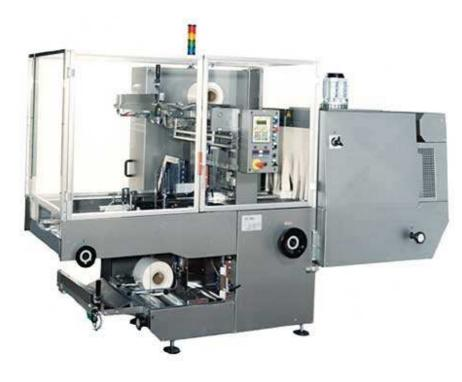
BFB MS500 collator stretch-banding machine for cartons.
