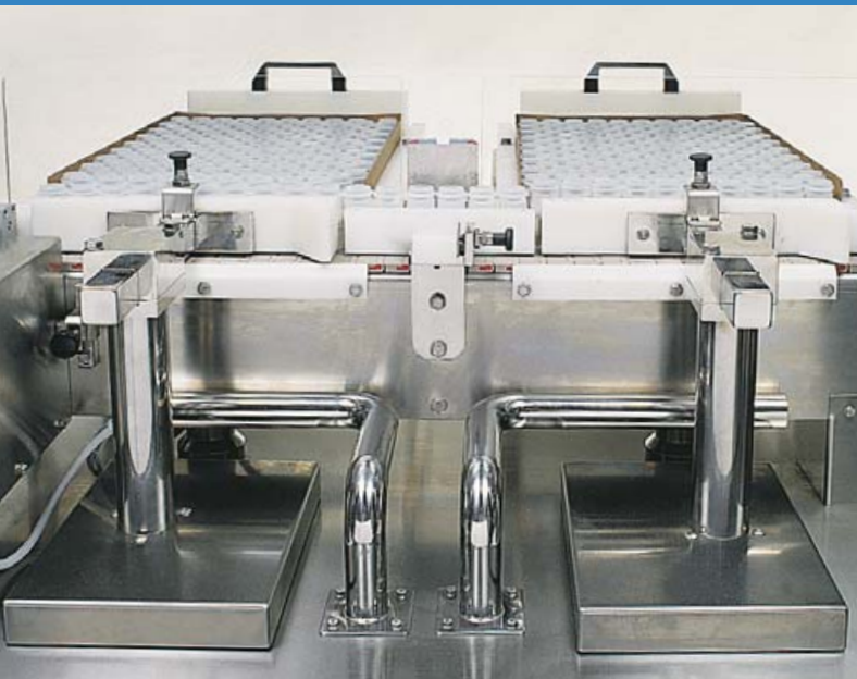
Tool-less change-over of vial size
