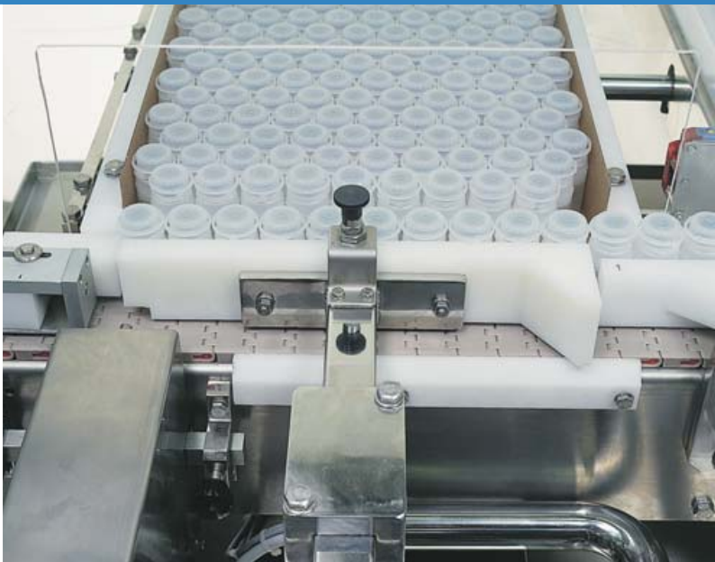
All mechanical movements are below the level of the vial mouths
