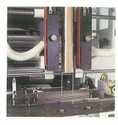
Elastomer jaw face acts as a cushion against shock for longer wear life. Jaw serrations are rounded which allows the film to float for
