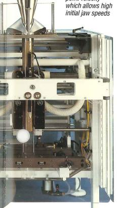
followed by a reduction to near-zero velocity at the jaw contact point to eliminate jaw slamming.
