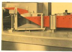
2. FORMER—After the roll stock passes through a scanner which detects registration marks on the web, it is then folded in half on a pivotal plow. This mechanism is designed to adjust for variations in winding and to help maintain the fold in proper alignment. In addition, a code dater or printer can be mounted on the machine at this station.
