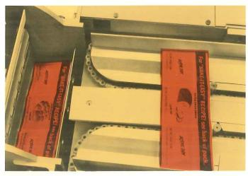
**PIN CONVEYOR**—Either double or triple serrated pouches are discharged from a knife vacuum drop off onto a right angle conveyor. Chain driven pin conveyors feed a predetermined count of pouches stacked either two, three or four high to a rotating transfer collection bucket.
