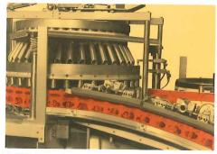
7. TOP SEALER—After leaving the filler, the strip of filled pouches is pulled through top sealer bars by power rolls to assure flat, wrinkle-free seals. High integrity seals, free of contamination, are provided by the natural arc of the closed web of filled pouches as it passes thru the top sealer. Excess air is expelled from the pouch before sealing.
