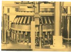
**4. VACUUM TRANSFER WHEEL**—The sealed pouches pass through driven rolls to the vacuum transfer wheel where the seals are positioned against "lands" which alternate with recessed areas. Vacuum, air and mechanics are used to open the pouch for insertion of the filling spouts.
