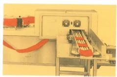
8. KNIFE—The continuous web of filled and sealed pouches is turned 90° and threaded into the rotary knife mechanism. The blades are mounted at an angle to provide shearing action for clean cutting. Single pouches or strips of perforated pouches can be placed onto a right angle or in-line discharge for further processing or transfer to Jones cartoning equipment.
