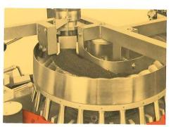
**6. FILLER**—The product is metered through an adjustable gate onto a rotating filler plate and is continuously proportioned into the spouts. This technique of gradual pouch loading avoids spout blockage and product flashback. The canted filler plate allows the spouts to enter the pouches and retract without reciprocating motions.
