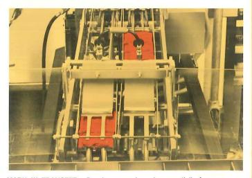
MARK III TRANSFER—Pouches are released sequentially from vacuum cups located on the rotary knife to form two lanes on a right angle transfer conveyor. Each group of pouches is shingled and accumulated on differential speed belts. Gates accumulate the stacks and discharge them into infeed buckets of an intermittent motion cartoner. For a constant motion Jones cartoner the transfer conveyor pivots in the direction of bucket travel during loading.
