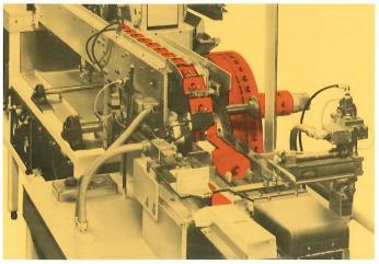
WHEEL STACKER—A continuous strip of filled pouches is cut on a rotary knife and transferred by vacuum cups onto a lug conveyor. The pouches pass through a conditioner to evenly distribute product for efficient collating. Pouches are collated by a stacker/counter and transferred into an indexing lug conveyor. Collected pouches are transferred to a loading station for automatic insertion into an end loaded carton.
