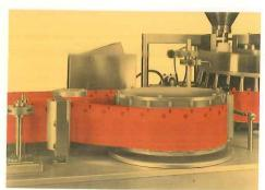
3. VERTICAL SEALER—The folded web is wrapped more than 180° around the vertical sealer to allow maximum dwell time for sealing into a continuous strip of individual pouches. The driven drum is equipped with cartridge heaters mounted vertically behind the seal bars. Packages with three- or four-sided seals can be made on the Pouch King.
