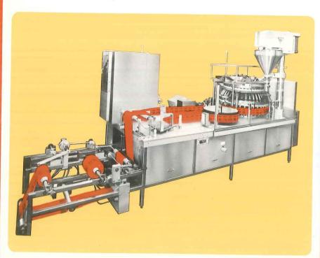
HIGH SPEEDS—Jones' continuous web concept keeps pouches under positive control during the Pouch King's high operating speeds. All rotary motion movements, including multiple station filling, sealing and cutting components, assure top performance and efficiency at highest speeds.
