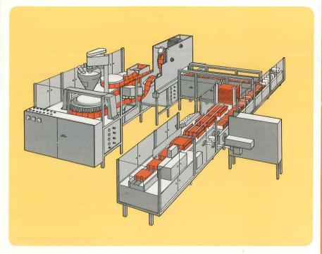
The form/fill/sealing of pouches on Jones' Pouch King machines is only part of the total story. Jones' expertise in package collating and cartoning is equally important for the integration of a reliable high speed packaging system.
