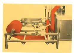
1. UNWIND—The unwind stand contains mandrels for mounting two pouch stock rolls, up to 24" (609 mm) diameter. The web travels over a dancer brake mechanism and variable speed rubber drive roll controlled by a signal from the photoelectric registration system. Automatic web splicers can be optionally provided.
