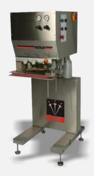
Retorquers are used after induction sealers to ensure the caps are correctly tightened after the induction sealer has melted the cap liner.
