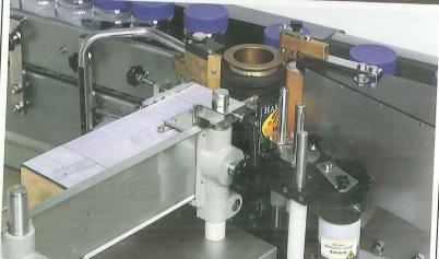
The well-proven labelling station of the KRONES ROTINA. The oscillating magazine is infinitely adjustable for different label sizes and positions.
