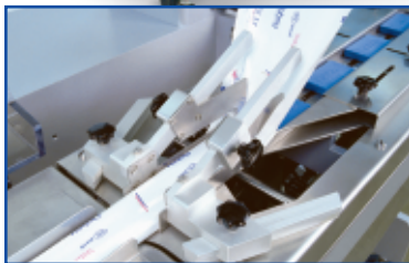
Adjustable Former Option, Fewer Parts for Faster Changeovers
