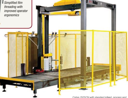
Cobra 1525CN with standard infeed, process and exit conveyor. Shown with Deluxe Fencing.
