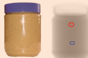
Peanut Butter Jar containing 1.2mm stainless steel and 3.0mm glass
