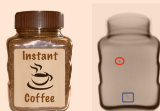
Jar containing 1.5mm stainless steel and 2.5 x 3 x 5 glass shard
