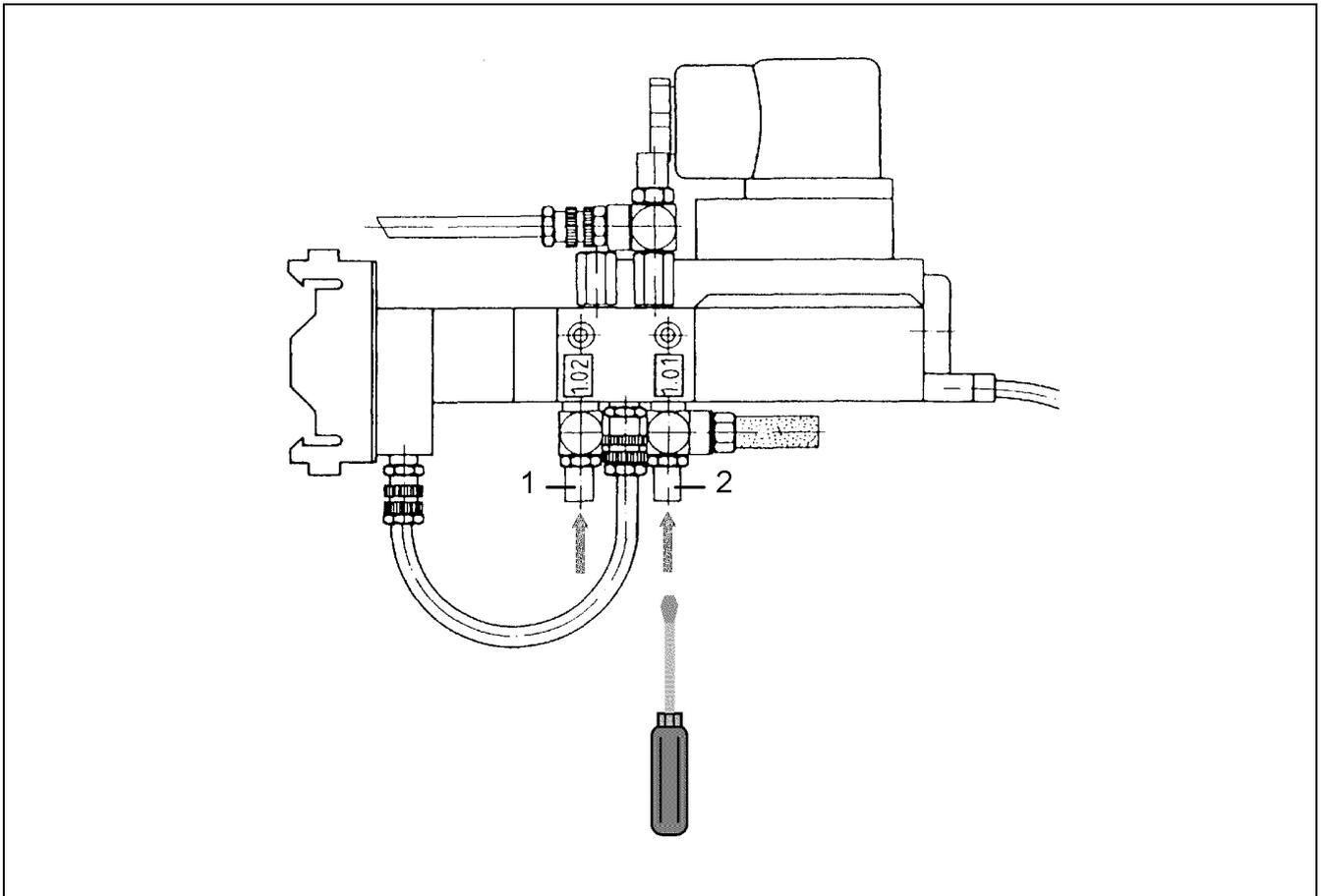
Figure 5: Adjusting the shutter speed
