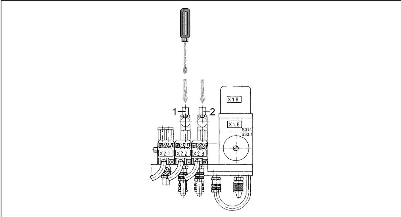
Figure 6: Adjusting the UV lamp cooling
