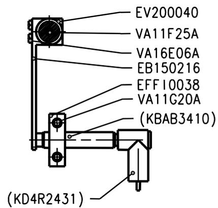
**Counter Pressure Cylinder, (Pos. E, XGA00002)**
