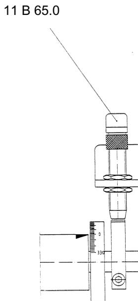
1. Turn the print image fine adjustor (see: print image positioning in longitudinal direction) in anti-clockwise direction until it stops.
