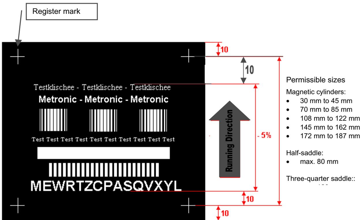
In order to patch the extension of the cliché mounted on the cylinder, at the vsk 400/410 the film-length is **reduced by five percent**.
