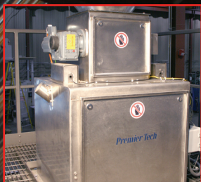
Stainless steel high speed gravity scale providing high precision weighing
