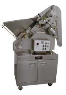
The Delta machines carrier links can be designed to fit one, two or four tablets per link depending on product size and printing requirements.
