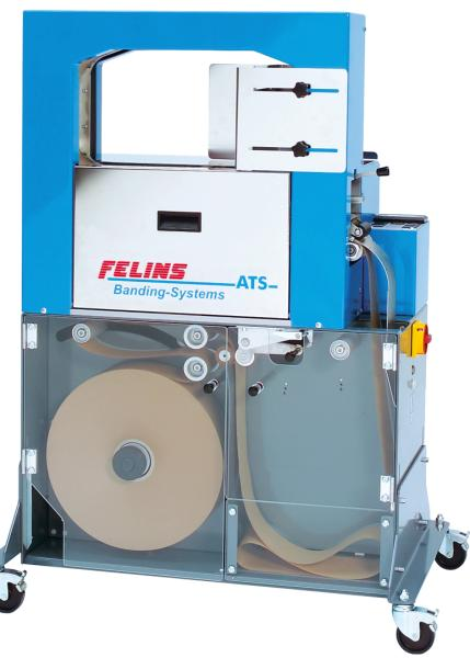
Felins offers the ATS US-2100 wide format bander, which is specially designed for band widths of 75mm and 100mm, respectively.
