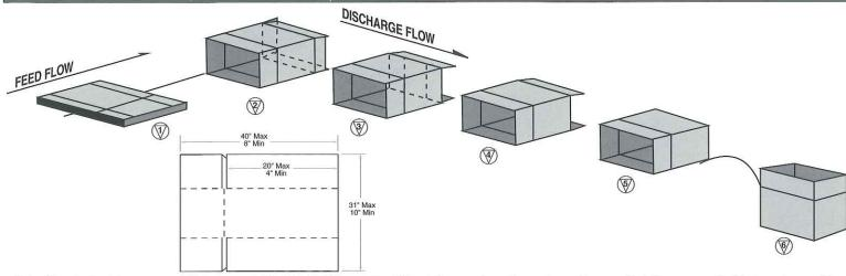
Note: A four inch minimum case width is required. The Model 201 is capable of the minimum and maximum shown. However, the full range, smallest to largest, cannot be realized on an individual machine.
