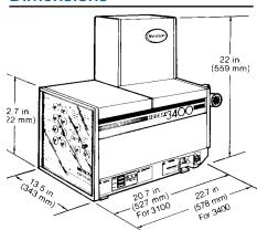
Dimension shown are for typical piston pump units. Gear pump units and units with OmniScan Control have different length and overall height measurements
