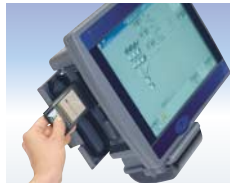
Memory Card Load product photos onto the operation screen to assist in selecting the correct product preset.
