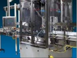
The TC Capper, shown with optional mirror-finish stainless steel, is available as a free-standing turret and in stand-alone or monoblocked configurations.
