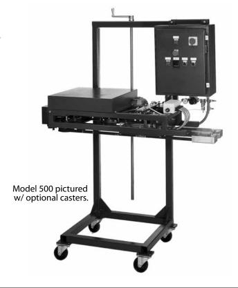
A unique hot air sealer produces a high quality "band type" seal on light mil bags (1.5–5mil). Perfect for ice, frozen foods, fresh foods, pet treats, birdseed, and other consumer packaging needs. DC variable speed control matches sealer to conveyor speed quickly and easily. Manufactured out of non-corrosive materials for use in damp or cold applications. Can be stand alone or integrated into a packaging line.
