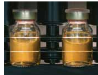
Special light to check albumin for microbial contamination
