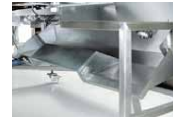
Bottom dust pan to collect dust, product debris and liquids in an easily accessible area
