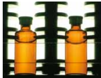
Background light in combination with Tyndall illumination
