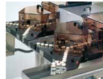
Y-Mag modules to separate two reject categories
