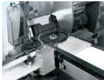
Infeed combination syringe/vial
