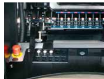
Push buttons for separate counting of rejects per defect group
