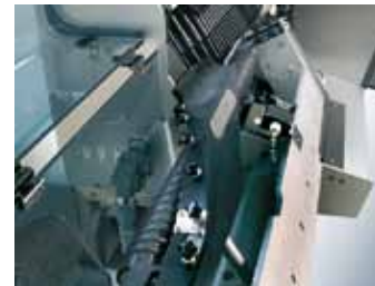
Syringe turning screw at infeed
