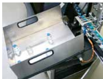
Separation of defects for bottles
